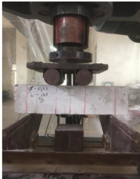
Figure 1. Flexural strength testing.
